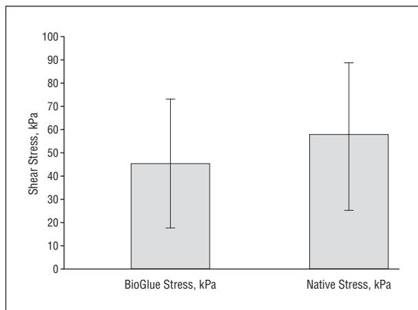
**Figure 3.** Comparison of shear strength values for native and BioGlue samples. The mean maximum shear strength values were obtained during testing for native and BioGlue Surgical Adhesive (Cryolife Inc, Kennesaw, Georgia) samples. There was no statistical difference between the native and BioGlue samples ( $P > .05$ ). Error bars indicate standard deviation.
