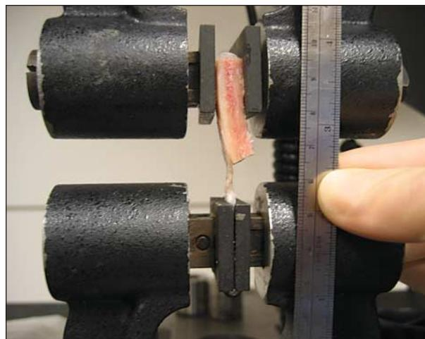
**Figure 2.** Bone and periosteum complex loaded into Instron Model 5500 (Instron Corporation, Norwood, Massachusetts).
